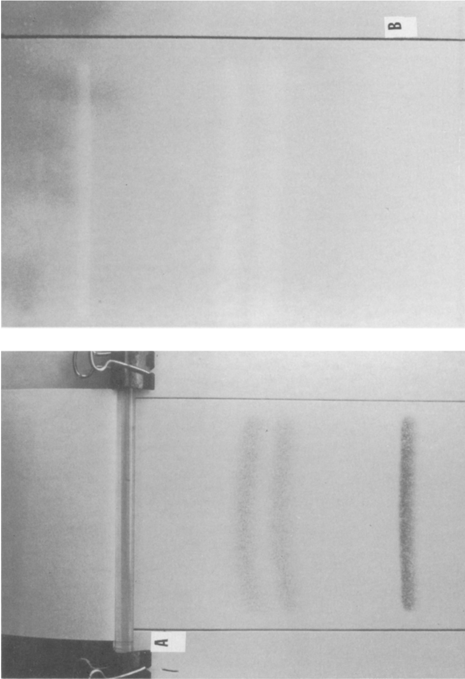
FIG. 2. Relative migration of deoxycholate (DC), chenodeoxycholate (CDC) and cholate (C) when subjected to continuous development thin layer chromatography (TLC). DC, CDC and C (500, 500 and 1000 \mu\text{g} ) were applied to 0.5 mm Silica Gel G plates, which were subjected to continuous development TLC using isooctane-ethyl acetate-acetic acid 100:50:14. Developed plates were sprayed with 2% \text{H}_2\text{SO}_4 in methanol (A) or with water (B) to detect bands. Mobilities relative to DC were 0.82 (CDC) and 0.17 (C).
