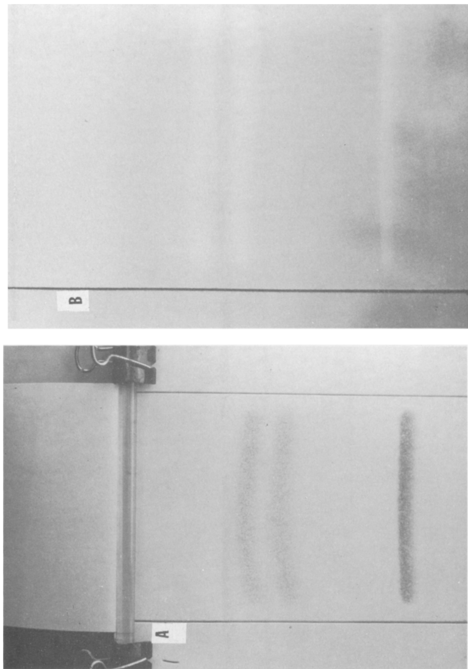
FIG. 2. Relative migration of deoxycholate (DC), chenodeoxycholate (CDC) and cholate (C) when subjected to continuous development thin layer chromatography (TLC). DC, CDC and C (500, 500 and 1000 \mu g) were applied to 0.5 mm Silica Gel G plates, which were subjected to continuous development. TLC using isoctane-ethyl acetate-acetic acid 100:50:14. Developed plates were sprayed with 2% H 2 SO 4 in methanol (A) or with water (B) to detect bands. Mobilities relative to DC were 0.82 (CDC) and 0.17 (C).
